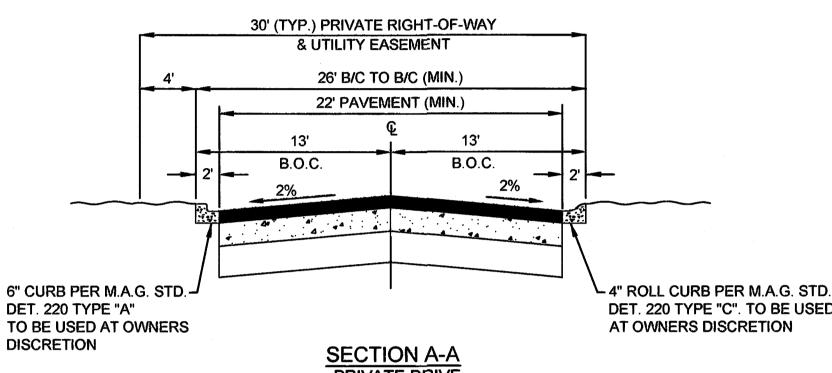
ALL PRIVATE DRIVES MAY BE CONSTRUCTED WITH INVERTED CROWN PAVEMENT AND/OR RIBBON CURB AT THE OWNER'S DISCRETION.
