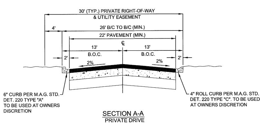
ALL PRIVATE DRIVES MAY BE CONSTRUCTED WITH INVERTED CROWN PAVEMENT AND/OR RIBBON CURB AT THE OWNER'S DISCRETION.
