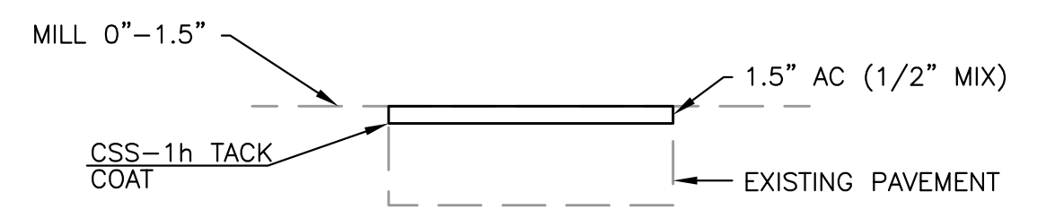
PAVEMENT STRUCTURAL SECTION NO. 3 NTS
