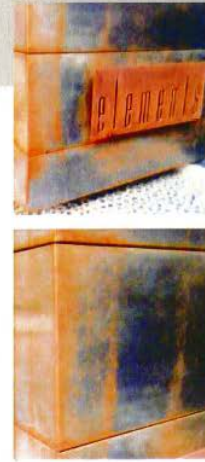
Element Metals unpolished sheet metal skin LRV=31 (oxidized patina shown above (color equivalency to Dunn Edwards Walrus)
