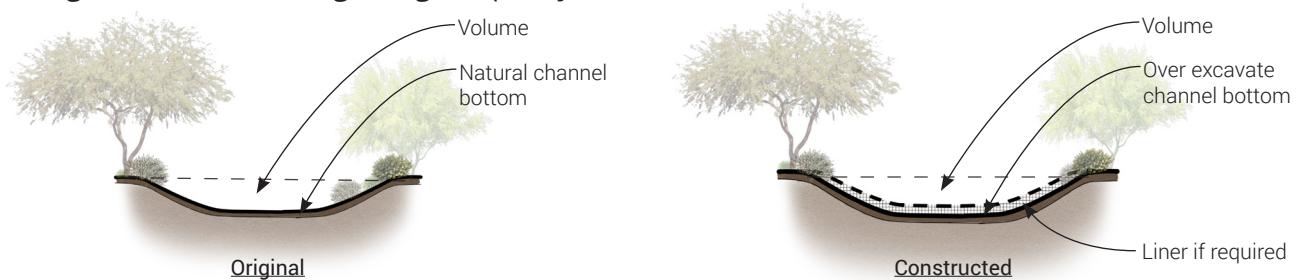
FIGURE 3.4 CHANNEL LINING DESIGN CAPACITY
