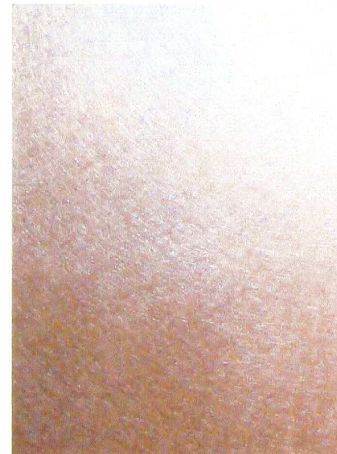
Element Metals unpolished sheet metal skin LRV=31 (oxidized patina shown above (color equivalency to Dunn Edwards Walrus))
