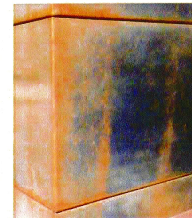
Element Metals unpolished sheet metal skin LRV=31 (oxidized patina shown above (color equivalency to Dunn Edwards Walrus))
