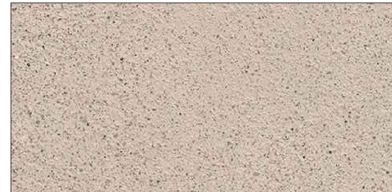
PRECAST CONCRETE - PARAPET CAPS AND TRIM: "OATMEAL", BY CDI, LRV: 28.71 TO MATCH EXISTING CONDITIONS
