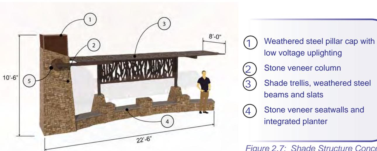
Figure 2.7: Shade Structure Concept
