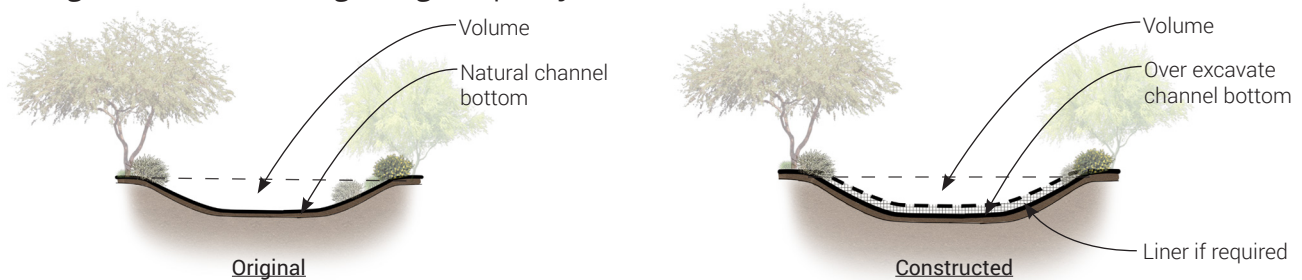
FIGURE 3.4 CHANNEL LINING DESIGN CAPACITY
