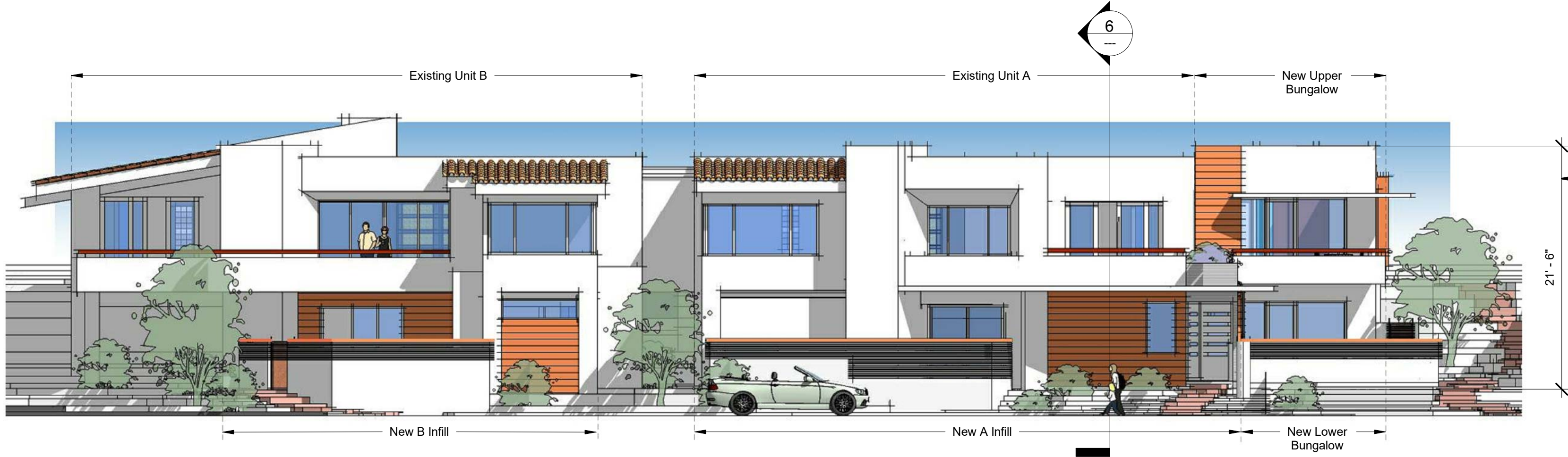
2 Typ. North Elevation with new Bungalows 1/8" = 1'-0"
