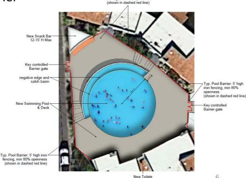
Typ. Pool Barrier: 5' high iron fencing, min 80% openness
