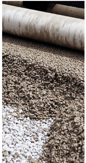
Porous concrete can reduce runoff sustaining in sidewalks and plaza areas.
