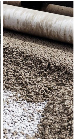
Porous concrete can reduce runoff sustaining in sidewalks and plaza areas.
