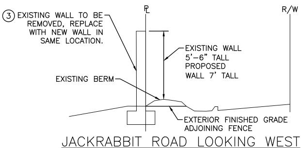
3 EXISTING WALL TO BE \( \tag{REMOVED, REPLACE} WITH NEW WALL IN SAME LOCATION. -EXISTING WALL 5'-6" TALL EXISTING — PROPOSED LANDSCAPING WALL 7' TALL BERMING -EXTERIOR FINISHED GRADE
