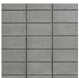
HONED BLOCK MASONRY
