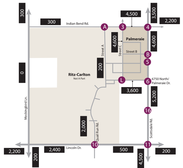
Figure 9: 2023 Site Traffic Volumes
